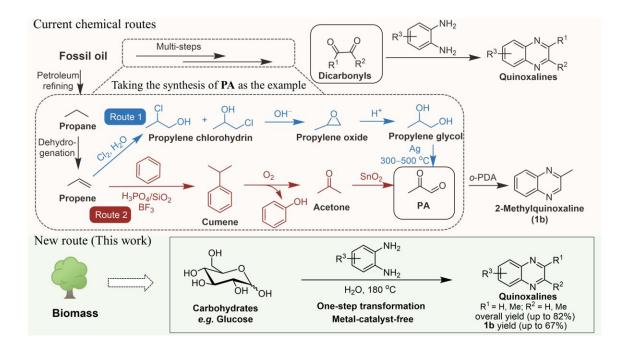
The upper part of the figure shows the current petroleum-based routes for manufacturing quinoxalines. The bottom part of the figure shows the proposed one-step sustainable approach based on biomass-derived carbohydrates. Credit: Science China Press
