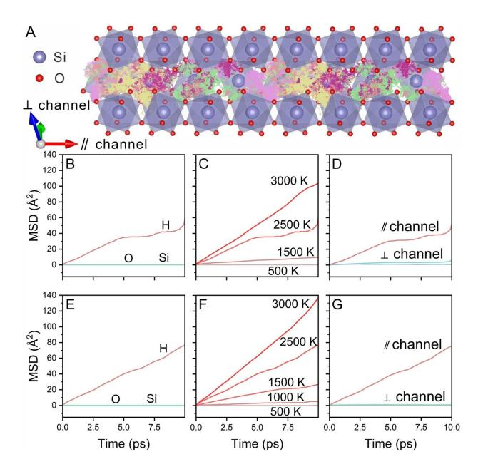
A) schematic plot for diffusive hydrogen (trajectories with various colors) in stishovite. B–G) calculated mean squared displacement at selected P-T conditions. Credit: *Science Advances* (2023). DOI: 10.1126/sciadv.adh3784
