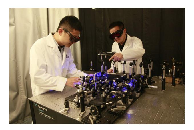
Researchers developed a diffraction-gated real-time ultrahigh-speed mapping (DRUM) camera that can capture a dynamic event in a single exposure at 4.8 million frames per second. Pictured are researchers Xianglei Liu and Jinyang Liang working on the optical setup. Credit: Xianglei Liu and Jinyang Liang, Institut national de la recherche scientifique (INRS)
