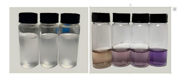
Left: solution containing cellulose extracted from sugarcane bagasse. Right: fibers in contact with material contaminated by glyphosate and submitted to the method for determining glyphosate levels at different pHs. Credit: Maria Vitória Guimarães Leal
