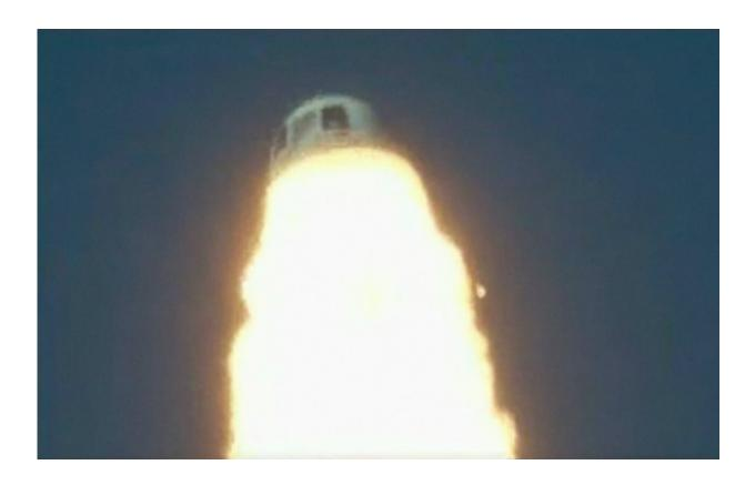
The report into the September 12, 2022 "mishap" said that failure of an engine nozzle caused by higher than expected engine operating temperatures caused the New Shepard rocket to fall back to the ground shortly after liftoff.
