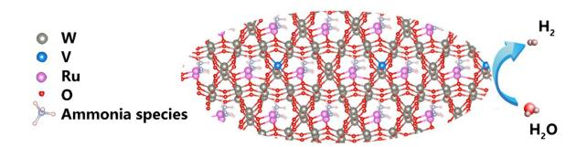
The atomically dispersed Ru is achieved in the hexagonal crystal channels of vanadium-doped tungsten bronze support via the precise coordination with channel ammonia, which exhibited highly efficient performance for hydrogen evolution reaction with remarkable mass activity in wide pH range. Credit: Chinese Journal of Catalysis
