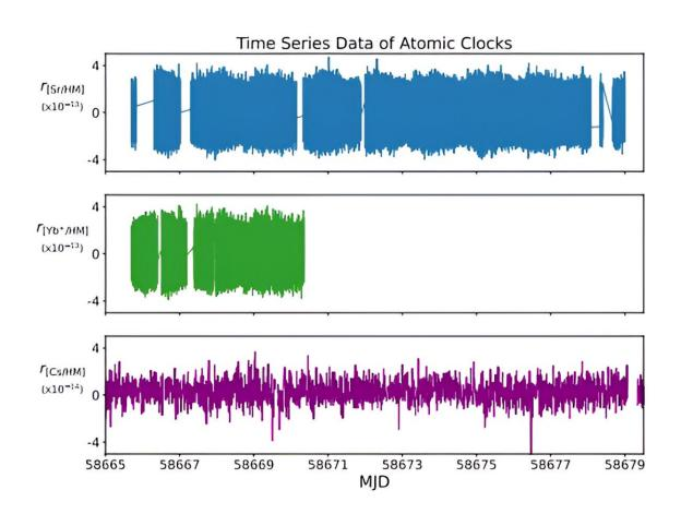
Top and middle: Fractional frequency ratios of Sr/HM and Yb<sup>+</sup>/HM data counted by NPL's femtosecond frequency comb, with data averaged over 1 s intervals. Bottom: Fractional frequency ratio of Cs/HM data produced by NPL's cesium fountain, NPL-CsF2, with data averaged over 600 s intervals. Data were collected between 1st and 14th July 2019 (MJD 58665–58679). Credit: *arXiv* (2023). DOI: 10.48550/arxiv.2302.04565
