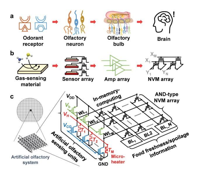
Biological olfactory system and proposed artificial olfactory system. a) Sequence of odor detection by the biological olfactory system. b) Sequence of gas detection by the proposed artificial olfactory system. c) Schematic diagram of the proposed artificial olfactory system. Credit: *Advanced Science* (2023). DOI:
