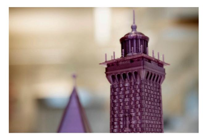
A 3D-printed model of West-Sweden's landmark, Vinga Lighthouse. The color of the material is determined by the metal used for the nanoparticles in the plasmonic plastic, as well as their shape and size. Credit: Chalmers/Malin Arnesson
