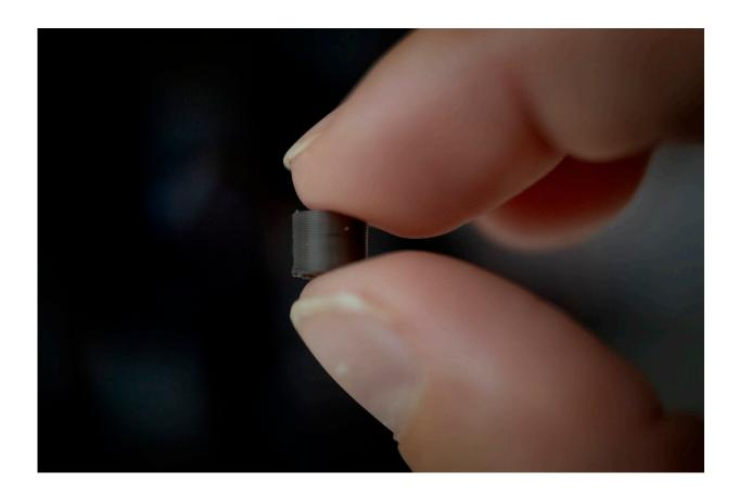
A filament of the plasmonic plastic. Due to its flexibility, the material can be formed into almost any shape. In this particular example, the filament is intended for use in 3D printers. Credit: Chalmers/Malin Arnesson
