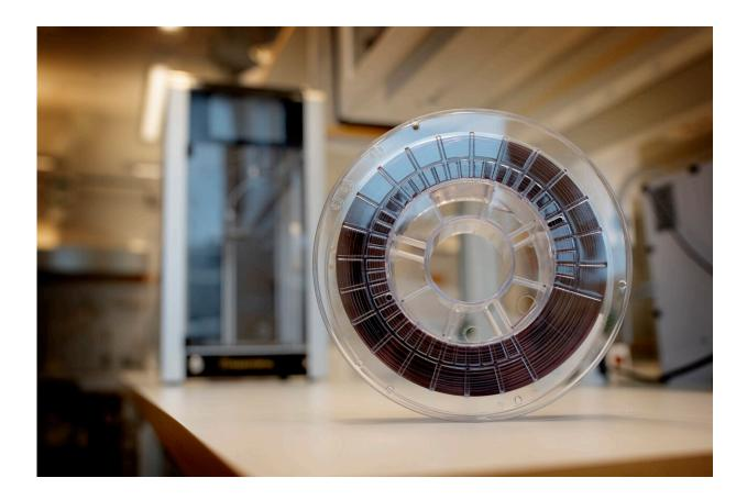
A 3D-printed sensing element made from plasmonic plastic for use in an optical hydrogen sensor. This particular element contains nanoparticles of the metal palladium, which gives it its gray color. Credit: Chalmers/Malin Arnesson
