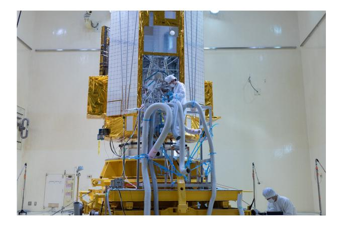
The XRISM spacecraft during acoustic testing at JAXA's Tsukuba Space Center in December 2022. These and other tests confirm that the spacecraft can withstand the severe vibrations and sounds of its rocket launch. Credit: JAXA
