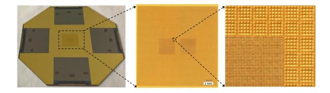
Figure 2: Zoom-in of prototype 100,000 -pixel magnetic calorimeter array showing the three different pixel types in this array. Credit: NASA GSFC
