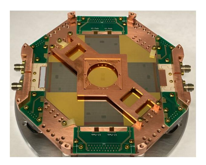
Figure 1: Prototype 100,000-pixel magnetic calorimeter array developed via collaboration between NASA GSFC and MIT Lincoln Laboratory. Credit: NASA GSFC
