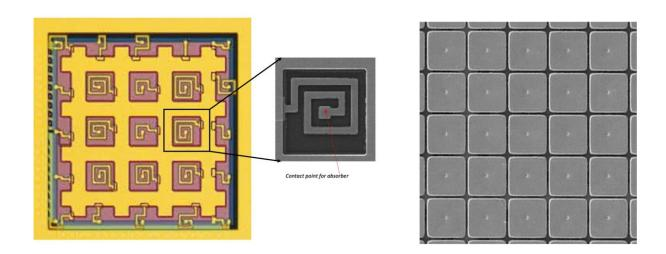
Figure 3: Photograph of a 25-pixel thermally multiplexed Hydra sensor. The waffle-shaped gold region is the magnetic sensor (left). The thin meandering lines emanating from the sensor are the different thermal links that go to 25 different contact points from which 25 independent X-ray absorbers can be suspended on top of the sensor, as shown in the electron micrographs (center, right). Credit: NASA GSFC
