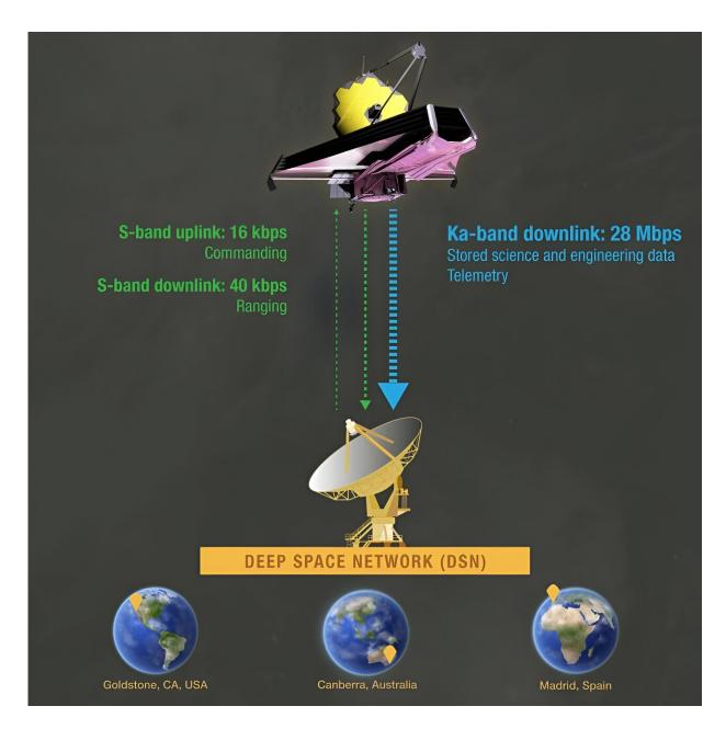
Webb talks to the Deep Space Network of antennas using S-band and Ka-band radio frequencies. For S-band communication, commanding instructions are uplinked at 16 kilobits per second (kbps) and observatory engineering telemetry and ranging are downlinked at 40 kbps. For Ka-band communication, stored science and engineering data and telemetry is downlinked at 28 Megabits per second. Credit: STScI
