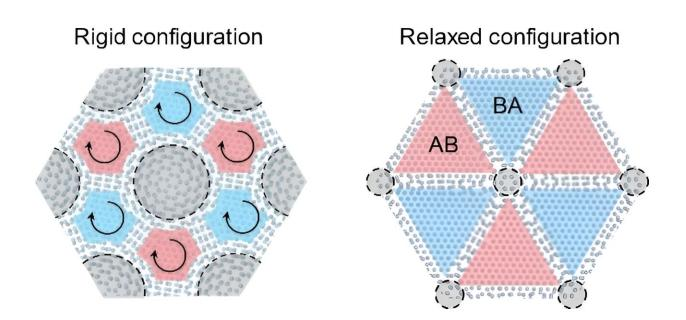
Schematics of the atomic structures before and after reconstruction of the twisted bilayer graphene. Credit: Science China Press
