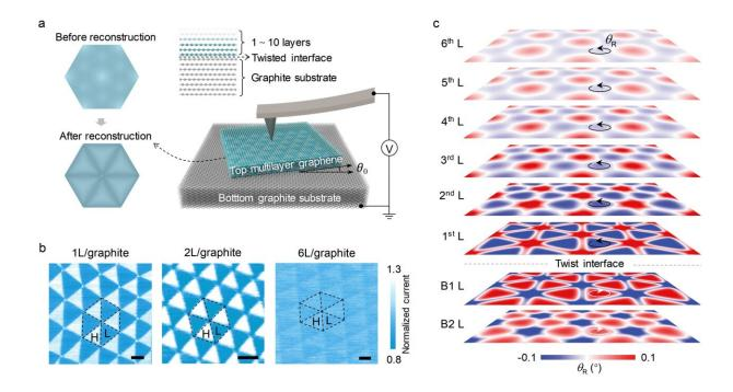
(a) A schematic of the experimental setup. (b) Typical current images measured on samples with twisted interface embedded in different depths. (c) Maps of the atomic deformation in individual graphene layers calculated by molecular calculations. Credit: Science China Press
