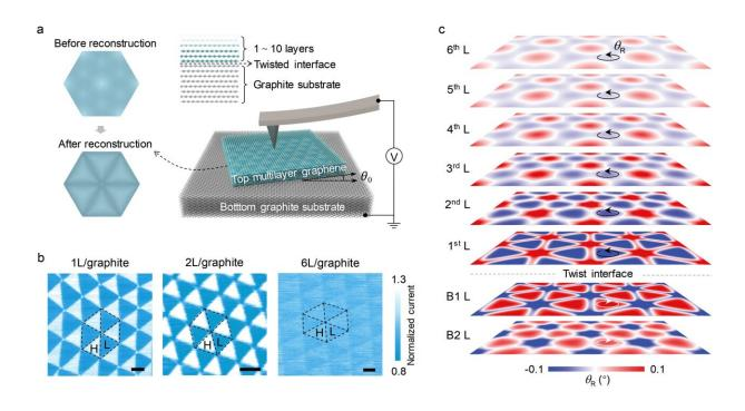
(a) A schematic of the experimental setup. (b) Typical current images measured on samples with twisted interface embedded in different depths. (c) Maps of the atomic deformation in individual graphene layers calculated by molecular calculations. Credit: Science China Press
