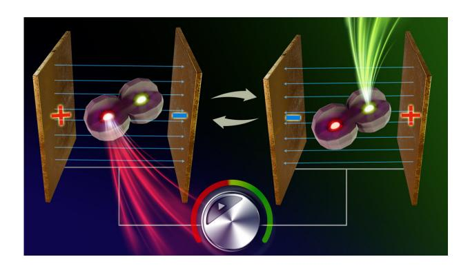
A nanoparticle made of two coupled quantum dots, each emitting light with distinct colors. applying an external voltage induces an electric field which can toggle the light emission from one side to the other, switching the emission color while keeping the overall light intensity. Credit: Artwork by Ehsan Faridi and Ehsan Keshavarzi—Inmywork Studio
