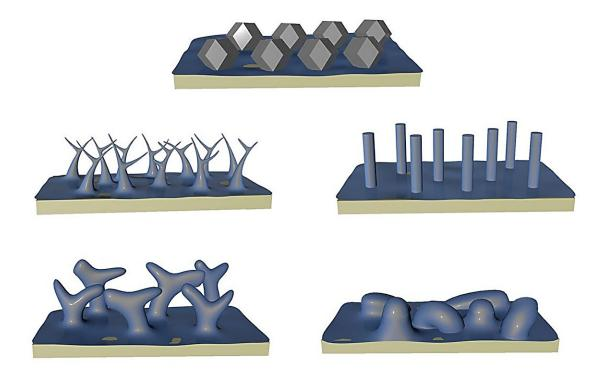
A rendering of the rhombic dodecahedron shape that lithium atoms formed on a surface with the researchers' technique for avoiding corrosion, top, with four illustrations (middle, bottom rows) showing the irregular shapes that appeared in conditions where corrosion formed. Credit: Li Lab/UCLA
