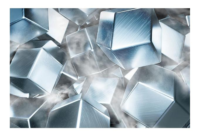
UCLA researchers developed a way to deposit lithium metal onto a surface while avoiding a layer of corrosion that usually forms. Without that corrosion, the metal takes a previously unseen form, a tiny 12-sided figure. Credit: Li Lab/UCLA
