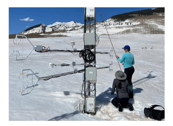
NCAR scientist Jacqueline Witte (kneeling) and software engineer Isabel Suhr (standing) measure the distance between sonic anemometer arms on an Integrated Surface Flux System (ISFS) weather tower. As the snowpack melts, they move the instruments down to stay close to the surface. This allows them to collect data on what happens to snow and water vapor at different levels in the air. Credit: Rosalyn Stilling, UCAR
