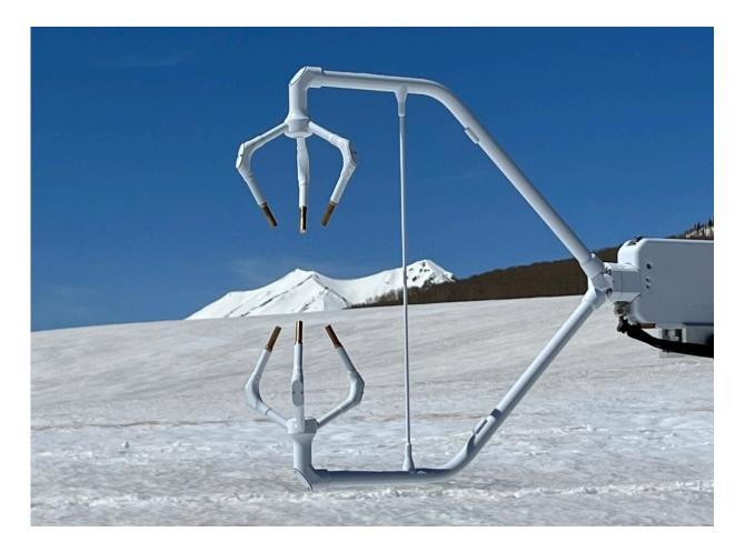
The three-pronged claws on this sonic anemometer are 3-D wind sensors that use sound to measure wind direction and speed. These measurements are vital for understanding exactly how sublimation occurs. Credit: NCAR & UCAR
