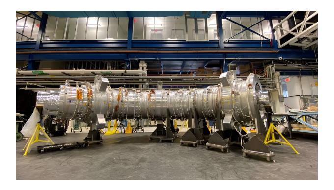
A segment of the Mu2e transport solenoid that will use superconducting magnets to focus roughly 10 billion muons per second onto an aluminum stopping target. Credit: Vito Lombardo, Fermilab
