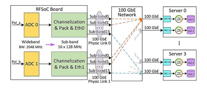
Architecture of UWB signal acquisition and processing system. Credit: XAO
