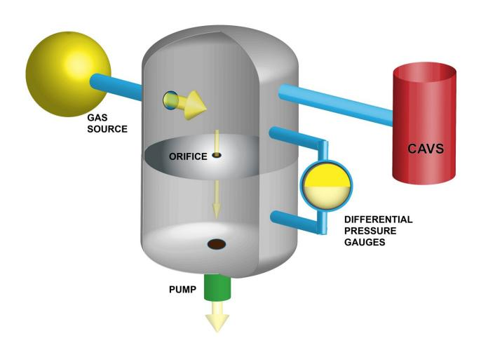
To verify the accuracy of their new approach for measuring ultra-low vacuum pressures, NIST researchers built a high-performance version of a traditional pressure metrology setup, known as a dynamic expansion system. In this system, they injected gas at a flow rate of roughly 10 to 100 billion molecules per second into the top chamber. The gas moved from the upper chamber to the lower
