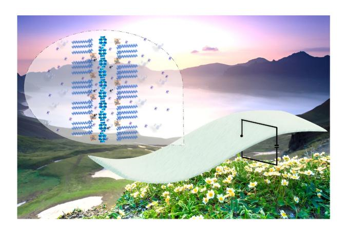
The polyoxometalate power generator collects the natural atmospheric humidity and produces continuous electrical signals by the uneven distribution and directional movement of ions, realizing efficient collection and utilization of low-value energy. Credit: Nana Research, Tsinghua University Press
