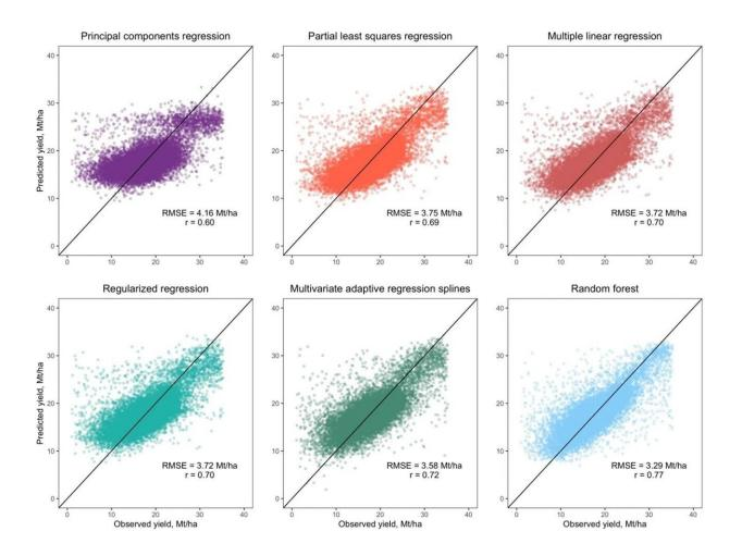
Comparison of machine learning model performances on test dataset (sample size = 4,800). Scatterplots for observed vs. predicted yields are shown. The solid line represents 1:1 relation between observed and predicted yields. Model comparison metrics shown are RMSE and Pearson's correlation coefficient (r). Credit: *Precision Agriculture* (2023). DOI: 10.1007/s11119-023-10057-1
