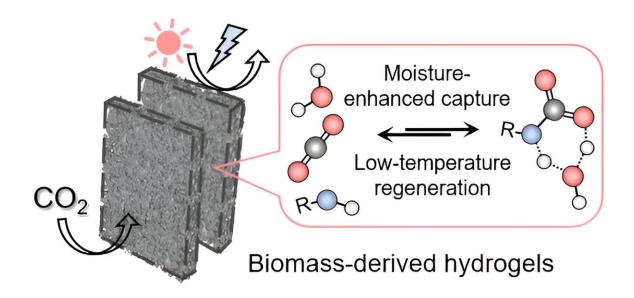
Fig 1. Schematic of the sustainable carbon capture hydrogels. Credit: Youhong Guo
