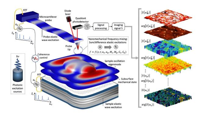
Schematic modalities where a probe (p), a sample (s), or both are excited by signals S of amplitudes a and adjustable frequency ω contents or coupled with specific properties of a specimen (e.g., photothermal or photoacoustic excitation by a photon of energy hυ). Credit: *Science Advances* (2023). DOI: 10.1126/sciadv.adg8292
