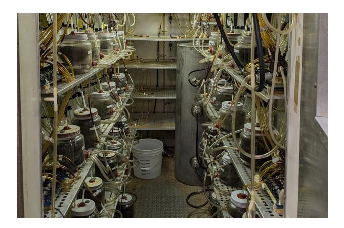
Inside this conditioned chamber in Rafael Auras' lab at Michigan State University, researchers can regulate composting conditions, including temperature, humidity and airflow, while measuring the carbon dioxide produced by microbes as they digest materials in the bioreactors. Credit: Matt Davenport/MSU
