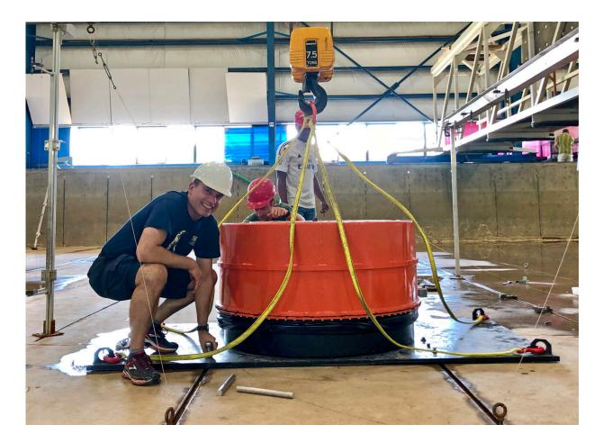
Hermann Fritz makes final preparations before the volcanic tsunami generator is installed in the wave basin at the Hinsdale Wave Research Laboratory at Oregon State. Credit: Georgia Institute of Technology
