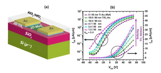
(a) Schematics of the fabricated  $MoS_2$  FETs, (b) measured transfer curves of the devices with series of  $TiS_x$  contact thicknesses, in both semilog and linear scales. Data for the reference sample is also provided. Credit: *Nanoscale Advances* (2023). DOI: 10.1039/D3NA00387F
