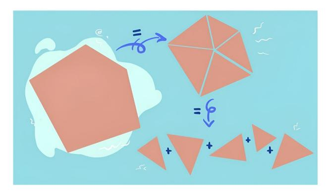
It can be easier to compute the area of a pentagon by chopping it up into smaller triangles. Credit: Maxine Calle, <u>CC BY-ND</u>
