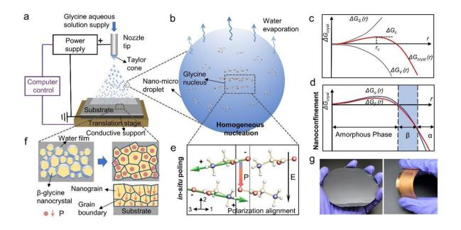
Fabrication and self-assembly mechanism of piezoelectric  $\beta$ -glycine nanocrystalline films. Credit: Springer Nature. *Nature Communications* (2023). DOI: 10.1038/s41467-023-39692-y
