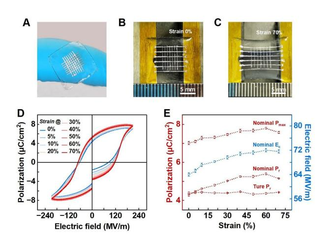
The elastic ferroelectrics under 70% strain. Credit: NIMTE
