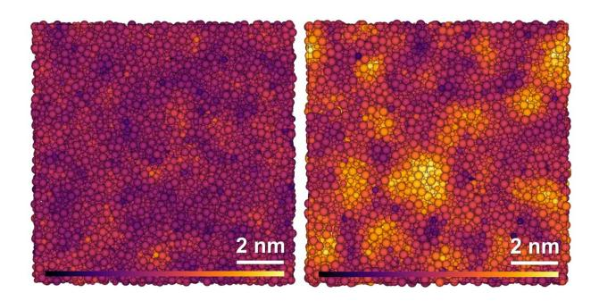
Simulated structure of glassy (left) and paracrystalline (right) grossular. The atoms of the elements oxygen, silicon, aluminum and calcium (from small to large) are coloured lighter the higher the degree of order in the surrounding structure. Credit: Hu Tang
