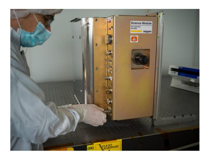
A member of the Cold Atom Lab mission team works on the Quantum Observer Module. The lab is a quantum science facility that's been operating on the International Space Station since 2018. This module is an upgrade to the lab's science capabilities. Credit: NASA/JPL-Caltech
