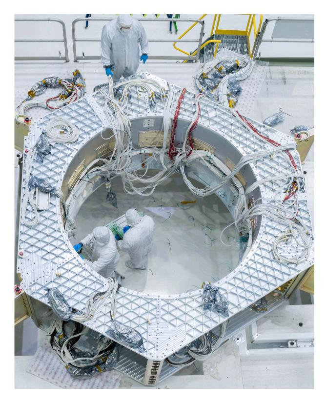
Technicians work to secure Roman's harness to the interior of the spacecraft flight structure. They are standing in the portion of the spacecraft bus where the
