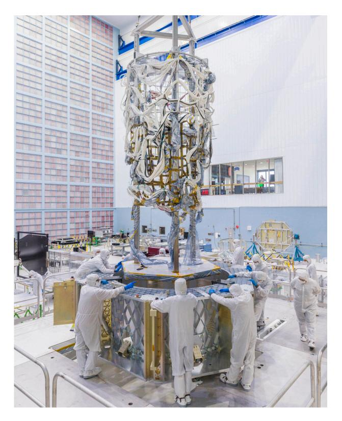
The Nancy Grace Roman Space Telescope's flight harness is transferred from the mock-up structure to the spacecraft flight structure. Suggested alt text: A
