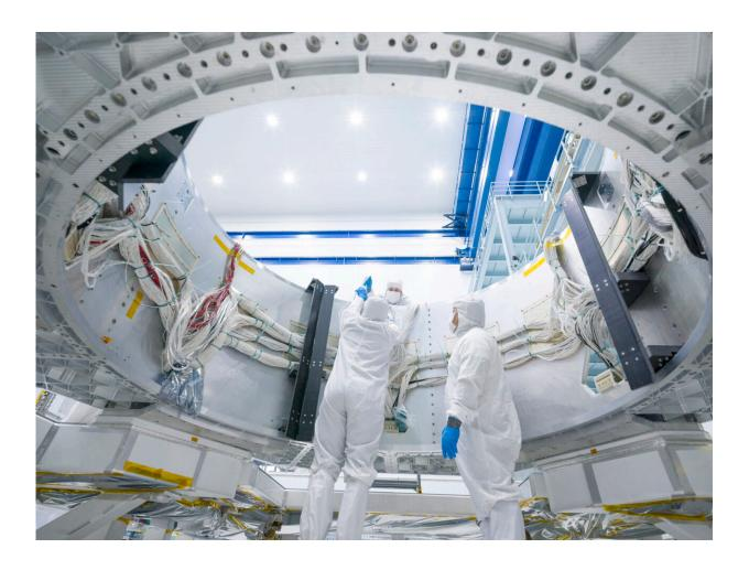
Technicians work to secure Roman's harness to the interior of the spacecraft flight structure. They are standing in the portion of the spacecraft bus where the
