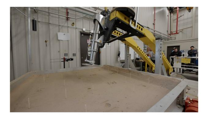
This setup is being used at JPL to test a 16-inch-diameter (40-centimeterdiameter) footpad for a future Mars lander. The footpad was plunged into a testbed filled with 10,000 pounds (4,536 kilograms) of simulated Martian soil in order to see how deep it would sink. Credit: NASA/JPL-Caltech
