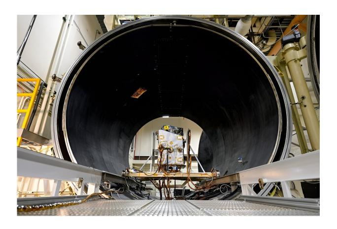
NASA's Lunar Trailblazer is shown here during thermal vacuum chamber (TVAC) testing at Lockheed Martin Space in Littleton, Colorado, in June 2023. Credit: Lockheed Martin Space
