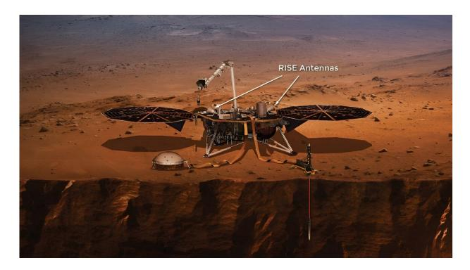
This annotated artist's concept of NASA's InSight lander on Mars points out the antennas on the spacecraft's deck. Along with a radio transponder in the lander, these antennas made up an instrument called the Rotation and Interior Structure Experiment, or RISE. Credit: NASA/JPL-Caltech
