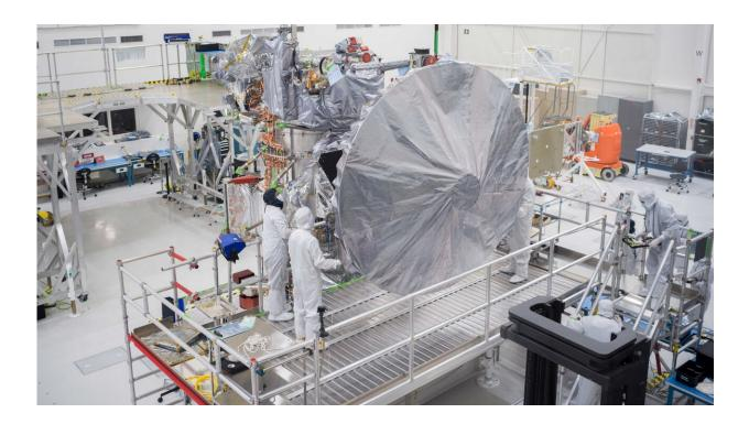
Engineers and technicians install Europa Clipper's high-gain antenna in the main clean room at JPL. Credit: NASA/JPL-Caltech
