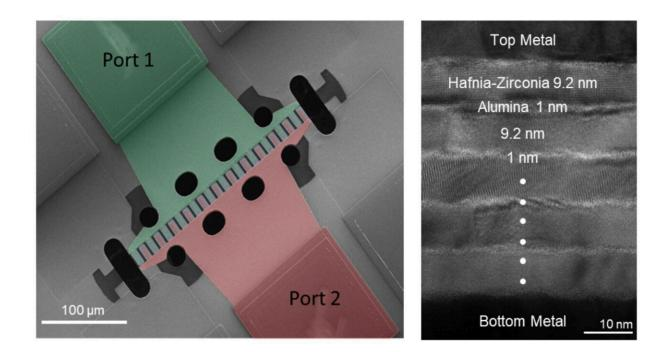
Scanning electron microscope of (left) hafnia-zirconia-alumina nanoelectromechanical resonator operating at 17.4 GHz and (right) resonator cross-section highlighting superlattice details. Credit: Tharpe et al.
