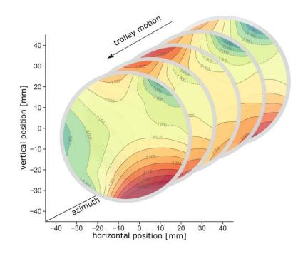
Typical magnetic field variations as mapped by the trolley at different positions in the Muon g-2 experiment's storage ring. Credit: Argonne National Laboratory.
