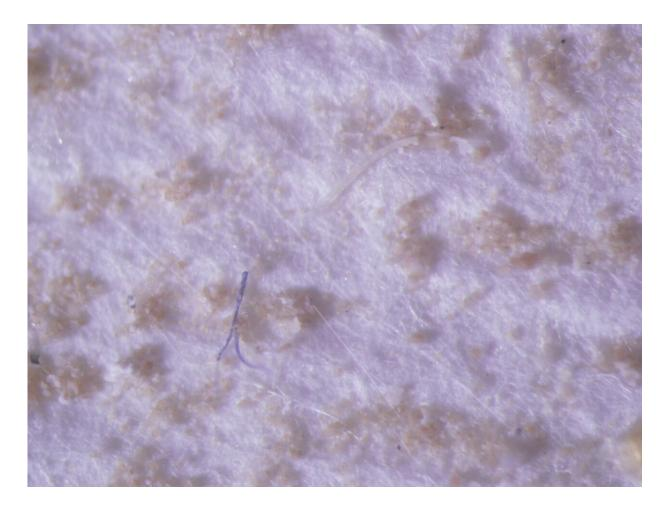
A blue microplastic fiber turned up on this glass fiber filter from the lung tissue of a beluga whale. Credit: Greg Merrill Jr., Duke University Marine Lab
