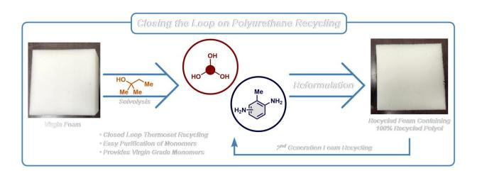
Researchers at Aarhus University have invented and patented a method to break down the chemical bonds in a polyurethane foam mattress and extract its monomeric building blocks. The polyol (the molecule in the red circle) can then be reformulated into a new PU foam mattress. Credit: Aarhus University
