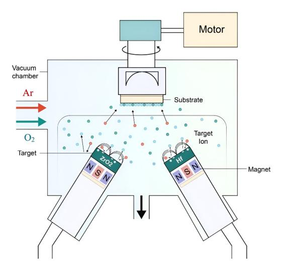
Deposition method of HZO layer. HZO layers of the TiN/HZO/TiN capacitor
