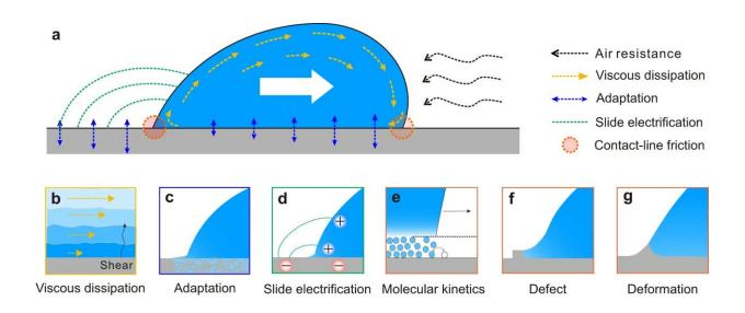
Schematic of all the possible effects contributing to drop friction. **a** A sliding drop is slowed down by the effect of air resistance, **b** viscous dissipation, **c** adaptation, **d** slide electrification, and contact-line friction due to **e** molecular kinetics, **f** defects, or **g** sample deformation. Credit: *Nature Communications* (2023). DOI: 10.1038/s41467-023-40289-8
