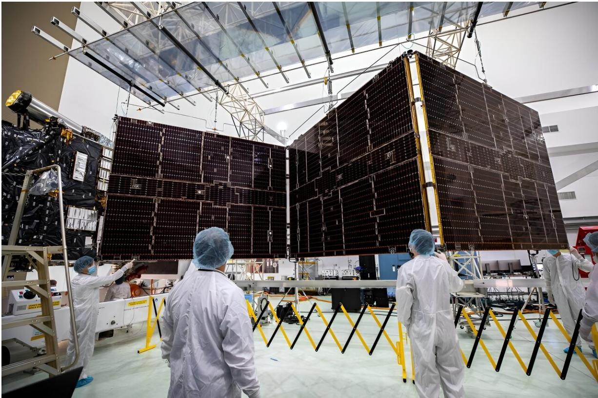
Technicians begin to retract one of the two solar arrays attached to NASA's Psyche spacecraft. This photo was taken on July 25 inside the Astrotech Space Operations facility near the agency's Kennedy Space Center in Florida. Credit: NASA/Kim Shiflett
