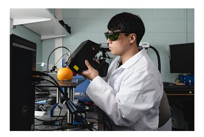
Purdue postdoctoral fellow Sungho Shin uses a portable LIBS spectroscopy instrument to collect data from the surface of an orange. Credit: Purdue University photo/Charles Jischke
