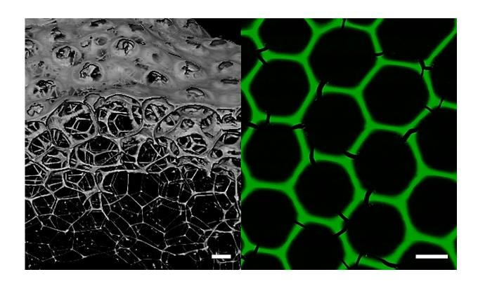
New biomaterials for industrial biocatalysis: Enzyme foams form three-dimensional porous networks with a stable hexagonal honeycomb structure. Credit: Julian Hertel, KIT
