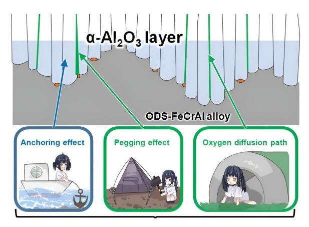
Fig. 2 Structure of  $\alpha$ -Al<sub>2</sub>O<sub>3</sub> layer and its functions. Credit: Assocaite Professor Masatoshi Kondo
