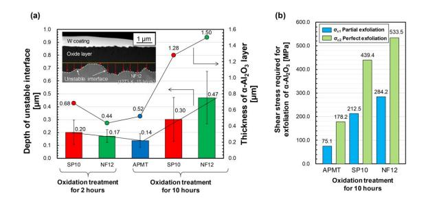
Fig. 3 (a) Relationship between  $\alpha$ -Al<sub>2</sub>O<sub>3</sub> layer growth and depth of unstable interface structure, (b) Shear stress required to detach  $\alpha$ -Al<sub>2</sub>O<sub>3</sub> layer. Credit: Associate Professor Masatoshii Kondo
