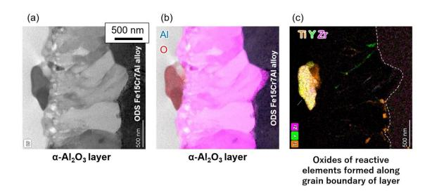
Fig 1 (a) Scanning transmission electron microscope image; (b) Energy dispersive X-ray (EDX) elemental mapping image of aluminum and oxygen; (c) Elemental mapping image of titanium, yttrium, and zirconium by EDX analysis. Credit: Associate Professor Masatoshi Kondo
