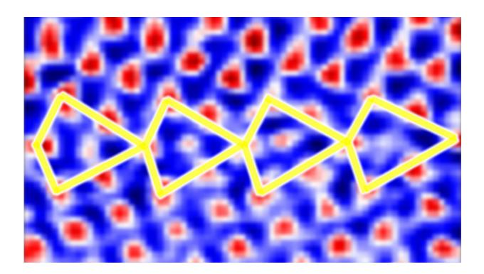
Transmission electron microscopy image resolving even light atoms (here: boron and carbon) as interstitial atoms in the centre of the atomic motif. Credit: Max Planck Society
