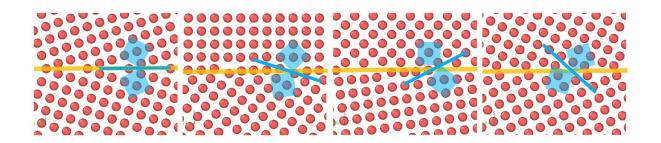
Even the mere tilt in the grain boundary plane with identical misorientation impacts the chemical composition and atomic arrangement of the microstructure and makes the material more or less prone to failure. Credit: X. Zhou, Max-Planck-Institut für Eisenforschung GmbH
