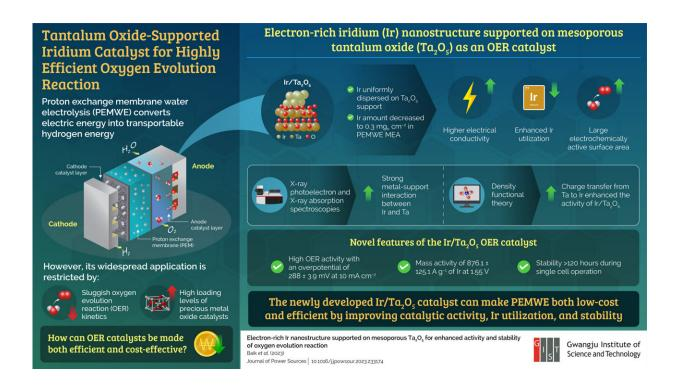
Researchers from Korea and USA develop a novel iridium catalyst with enhanced oxygen evolution reaction activity, facilitating a cost-effective proton exchange membrane water electrolysis for hydrogen production. Credit: Chanho Pak from Gwangju Institute of Science and Technology
