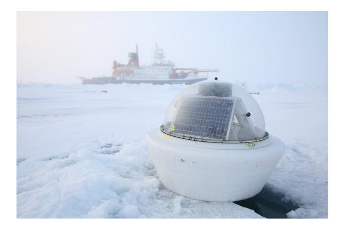
Scientists install buoys on an ice floe in the Central Arctic Ocean at the end of the MOSAiC leg five with RV Polarstern in September 2020. The buoys are working as an autonomous bio-physical observatory on sea ice and in the ocean.
