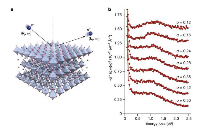
High-energy M-EELS spectra from  $Sr_2RuO_4$ . **a**, Conceptual illustration of reflection M-EELS experiments from a cleaved  $Sr_2RuO_4$  surface. **b**, Fixed-q (in r.l.u.) energy-loss scans for a selection of q values along the (1,0) crystallographic direction, taken at T = 300 K. These spectra were obtained by dividing the M-EELS matrix elements and scaling the curves as described in ref. <sup>37</sup>. At small momenta (q
